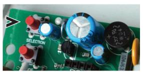
Press & hold bottom button. Release when door is fully open.
