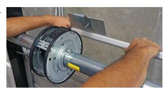
Release (undo) brake cable handle completely. The motor can now rotate by hand.
