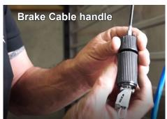
Set closed position. Move white adjuster until it touches the small red switch contact.
