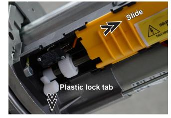
3 Undo cable to releaser brake.
