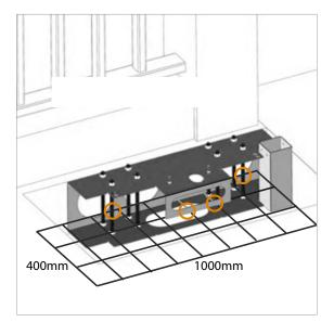
2. Tie the reo to the Slab at the points circled in orange shown above
