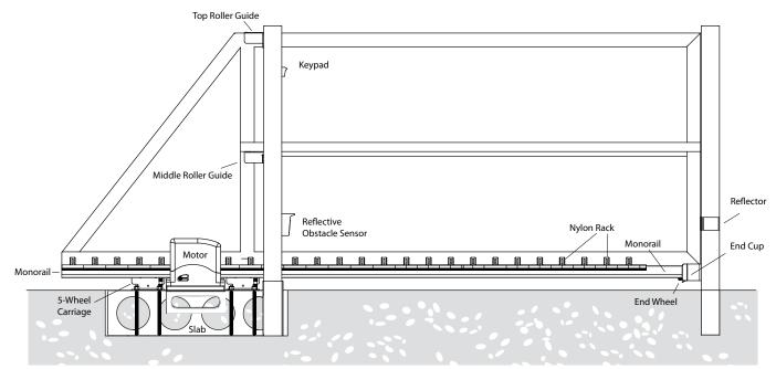
Cantilever driveway gates are far superior to rolling track systems. The gate never jumps off the track, because there is no track.
